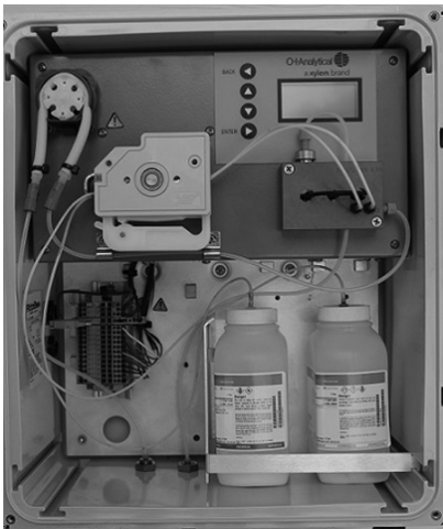
Figure 7: Sample pump shown with cover off
